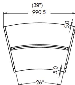
The Frontline end panel has a 0.16" (4 mm) flat front edge of solid wood. The distance between the front edge of the end panel and the front edge of the shelf is 0.02" (5 mm).
